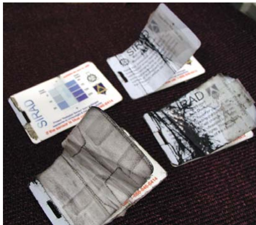
Figure 3. Photo of damaged SIRADs returned at the end of field deployment. For one of the dosimeters, the protective cover was entirely missing, and for the others, the cover was not held flat, leaving the sensitive strip unprotected from light.
